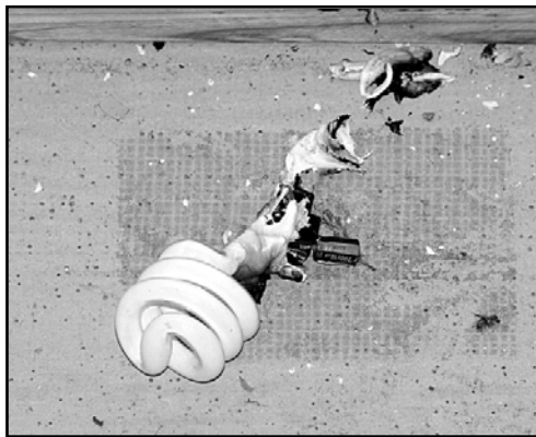
Figure 13. Remains of helical CFL on floor. Glass tube and electronic components are mostly intact.
