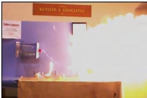
g) Expelled fluid separate from vessel.
