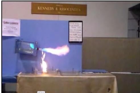
c) Fluid beginsejection as flame enters vessel.
